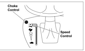
Figure 16. Independent Speed and Choke Controls
